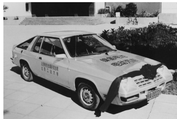
Fig. 5. The first EVs in China driven by Ni/MH batteries.
